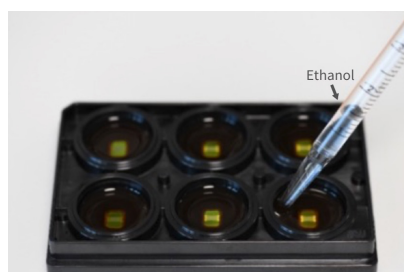
Figure 2: Filling the Wells of MaxTwo Multi-Well Plate with 70% Ethanol
